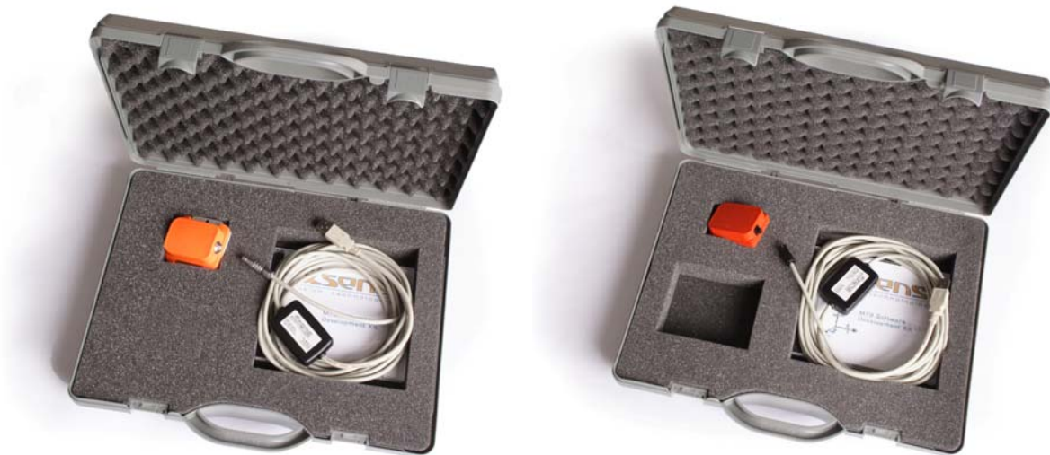
Photos of the MTi (left) and MTx (right) Development Kit
